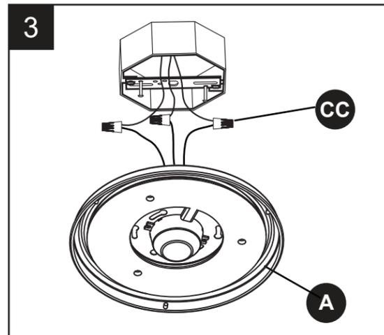
4. Lift fixture pan (A) up toward ceiling and carefully tuck wires into outlet box. Align keyholes on fixture pan (A) with long screws (BB), then twist fixture pan (A) until the long screws (BB) engage the narrow end of the keyholes. Tighten long screws (BB) to secure.
