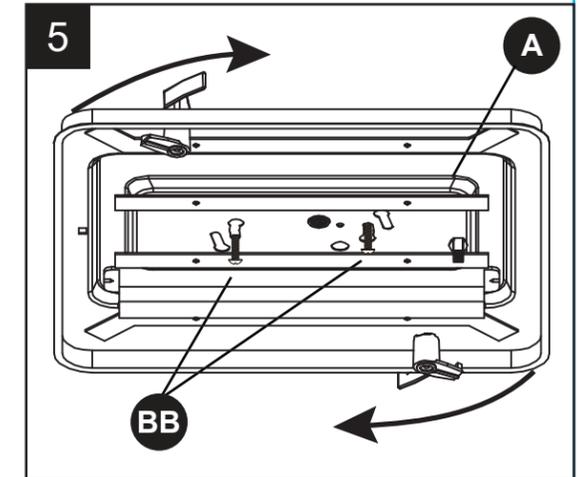
6. Align the diffuser (B) over the fixture plate (A) and gently close the two diffuser locks by turning the levers in towards the fixture. Ensure that the diffuser is fully supported and secured to fixture plate before releasing and completing the installation.
