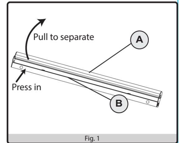
2. There is no need to disconnect the two halves of the fixture body. Support cables will support the weight of the LED cover assembly (A) during positioning of the housing base (B) up against the mounting surface.
