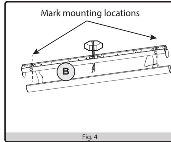
4. **DRYWALL MOUNTING:** If the mounting holes go through drywall without a stud, drill two small pilot holes using a 3/16-in. drill bit (not included), and install drywall anchors (AA) into the holes with a hammer (not included).
