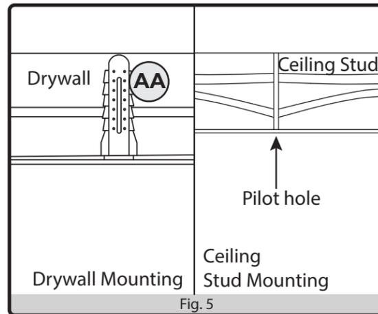
**CEILING STUD MOUNTING:** If the mounting holes go through ceiling studs, drill four small pilot holes using a 5/32-in. drill bit (not included) for the wood screws (BB).
