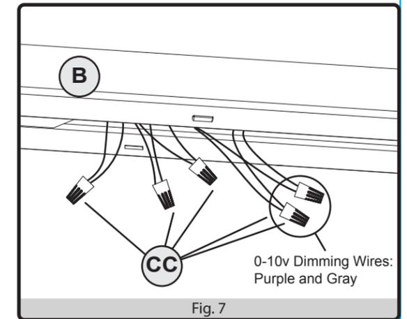
6b. **If the fixture is configured with an emergency battery back-up system:**
