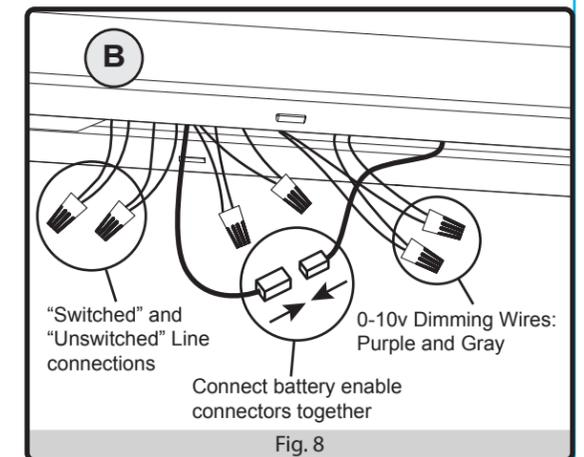
7. Tuck all loose wires and cables into the housing base (B). Gently press housing base (B) near one end of the fixture while securing the LED cover assembly (A) until all latches securely engage with the housing base (B).
