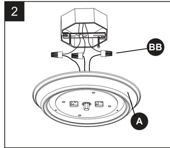
3. Lift fixture pan (A) up toward ceiling and carefully tuck wires into outlet box. Align keyholes on fixture pan (A) with long screws preassembled on crossbar (AA), then twist fixture pan (A) until the long screws engage the narrow end of the keyholes. Tighten long screws on crossbar (AA) to secure the fixture to ceiling.
